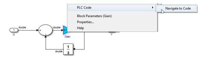
**2** Selecting **Navigate to Code** activates the HTML code generation report. The following figure shows the result of tracing the Gain block within the subsystem.
