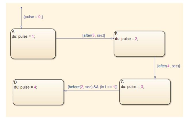
You can map states and transitions in the chart to the generated code. For instance, the transition from state B to C appears as:
