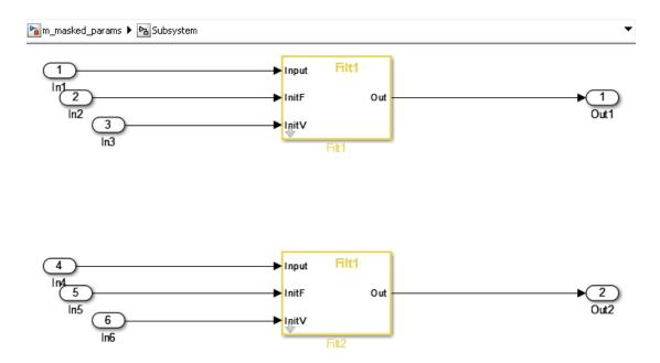
The two subsystems, Filt1 and Filt2, have different values assigned to their mask parameters. In this example, Filt1\_Order\_Thau is a constant with a value of 5.
